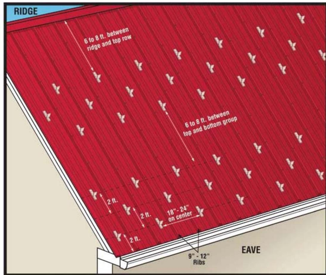
Horizontal spacing will be dictated but how far apart the metal seams or ribs. Shown is a typical RTMINI application on a 9" or 12" center rib panel. Do not place Snow Guards beyond the bearing wall on an extended roof section. Please see Appendix page A7 for general installation information.
