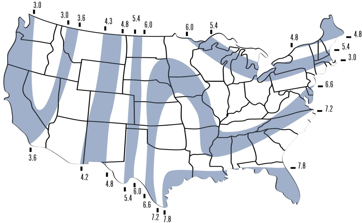
Rainfall intensity is measured in inches per hour. Capacity of residential gutters should be planned to handle the most intense five minute burst of rain that is likely to occur. Find the maximum rainfall intensity for your area on the map.
