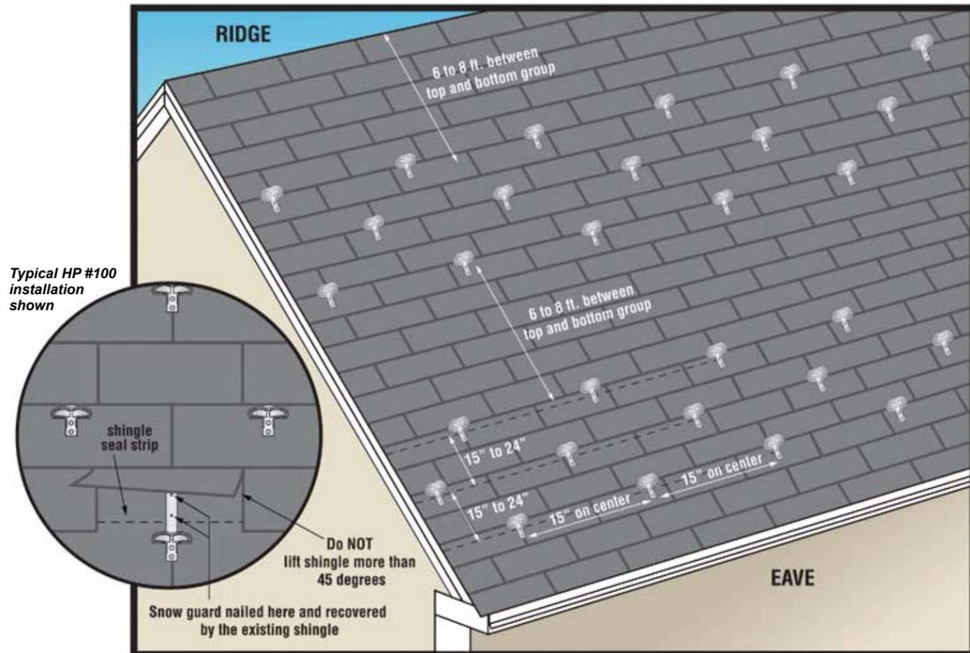
Do not place Snow Guards beyond the bearing wall on an extended roof section. Appendix page A7 for general installation information.
